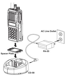
1) The VAC-UNI (CD-58/PA-55) charges only the Vertex Standard FNB-V127LI-UNI, FNB-V128LI-UNI and FNB-V129LI-UNI Lithium-Ion Battery Pack.
