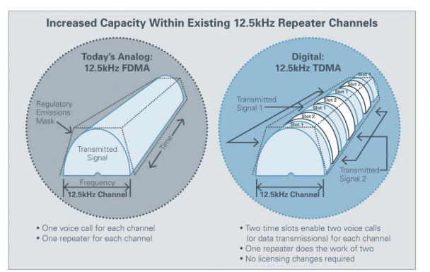
When FDMA technology is used to split a channel into two subchannels, the resulting signals must still fit within the channel's required emissions mask
