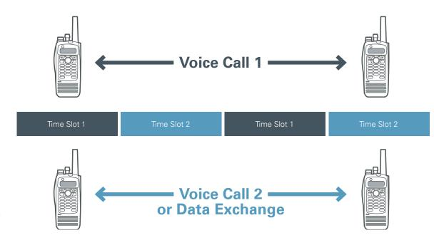
TDMA divides a 12.5 kHz channel into two alternating time slots to achieve 6.25 kHz equivalent spectral efficiency when used with a repeater.
