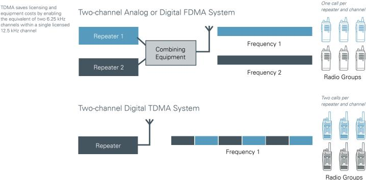
equipment costs by enabling the equivalent of two 6.25 kHz channels within a single licensed 12.5 kHz channel
