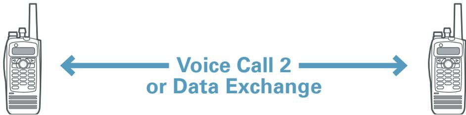
TDMA divides a 12.5 kHz channel into two alternating time slots to achieve 6.25 kHz equivalent spectral efficiency when used with a repeater.
