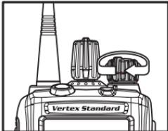
A line drawing of the top panel of a Vertex Standard transceiver. The VOL/PWR knob is shown being turned clockwise. The device has an antenna on the left and a display screen on the front.
