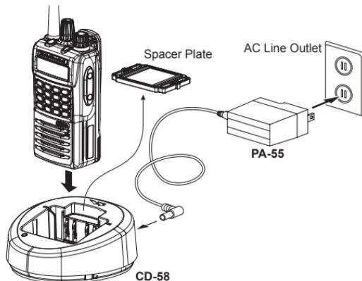
proper positioning of the battery pack. If charging with the transceiver attached, turn the transceiver off. The antenna jack should be at the left side when viewing the charger from the front.
